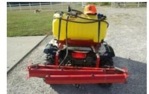
Most sprayers now have the two-wire plug in making it very fast to hook power to the pump. The version pictured has a direct hookup to the battery.
