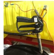
The 25 gallon version shown here, allows us to spray two (2) acres easily and does not upset the center of gravity of the ATV. Mount the sprayer on the rear rack of the ATV. Use two (2) tie-down straps to keep the unit steady and in place. Placing a towel under the sprayer unit will keep it from scratching the racks. Rubber strips also work well.
